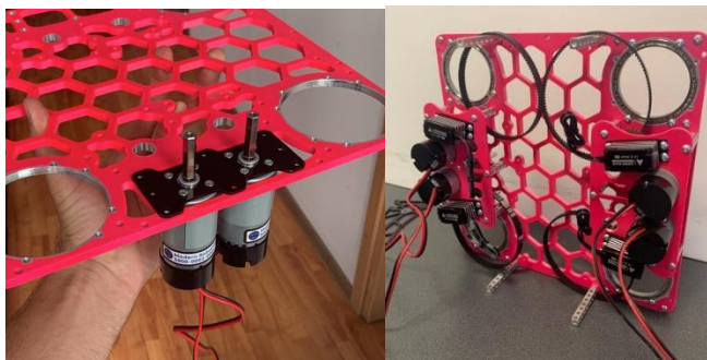
Figure 24. Left – Motors are mounted; Right – Servomotors are mounted.
