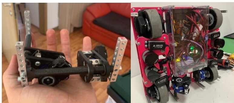
Figure 27. The odometry subassembly
