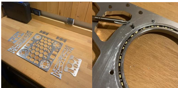
Figure 21. All CNC parts produced and a failed tap.
